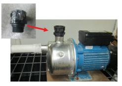
**Step 4:** Thread Wizard assembly to the BARREL UNION/pump outlet.
