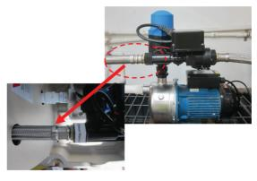
**Step 7:** Install a filter between the tank and tank inlet. This ensures that clean water is supplied to the pump.
